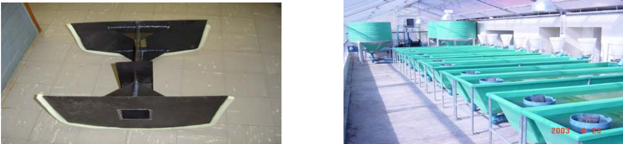
Figure 1: Two-chamber test compartment and experimental system 10 x 25000 litre recirculation raceway system.
