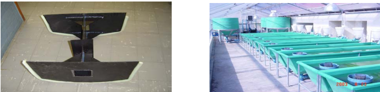
Figure 1: Two-chamber test compartment and experimental system 10 x 25000 litre (m 3 ) recirculation raceway system.
